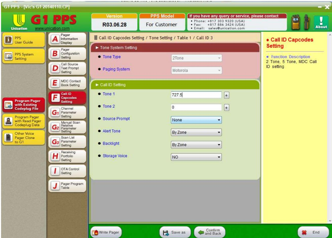
Now, when one goes to enter Tone 2's frequency note below what happens to Tone 1's value, it changed to 726.9 (see below screen shot). This adjusted value is well within the tone frequency generation accuracy of any current paging encoder (e.g., Zetron) and should not be a problem. However, if one needs to manually enter the frequency 727.5 for another tone pair or Long tone they will have to enter the 726.9 value or the programming software will display a "Tone Frequency Error"
