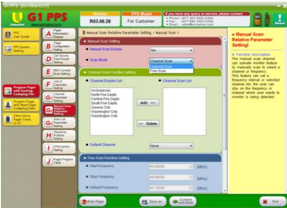
To enable a scan list set **Manual Scan Enable** to **Yes**. Then select in the **Scan Mode** field either **Channel Scan** or **Free Scan**. Each mode is reviewed below.
