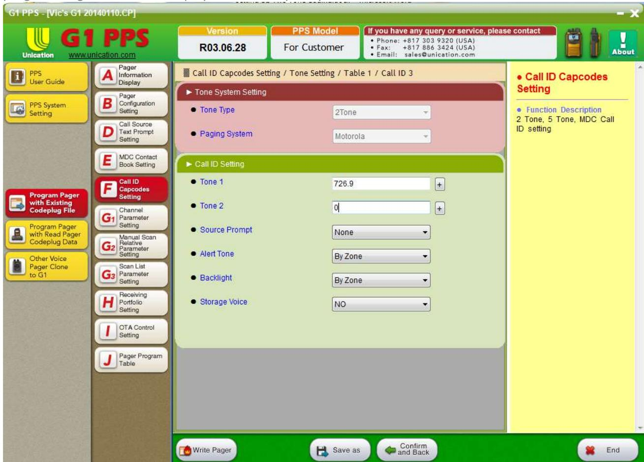
It is important to note that a Tone Table is not limited to just the tone frequencies of the selected Paging System (e.g., Motorola, GE, etc.), but when doing this it is possible the tone frequency entered may be adjusted. It is this adjusted value that needs to be manually entered for other tone pairs (or Long tones) that use this tone frequency.
