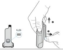
After the belt clip is assembled to the radio, you can wear the radio to a certain fixture (such as a belt). The belt clip is designed with a buckle to ensure the fixing performance. To take out the belt clip, press and hold the buckle in the direction as arrow ① shows and lift up the belt clip in the direction as arrow ② shows. See the figure above.
