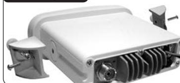
3. Attach the mounting brackets to the sides of the transceiver with the adjusting screw flanges facing the back of the flat surface.
