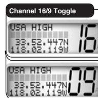
To exit the **Channel 16/9** mode and return to the previous channel, press and hold the **Channel 16/9** button.
