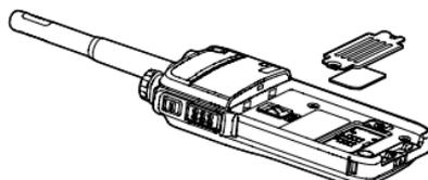
Step 3 Replace the cover and tighten the screw as shown in the figure below.
