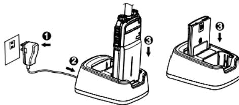
The charger LED indicates you the charging process. When the charger LED glows red, the charging begins. When charging is complete, the charger LED glows green.
