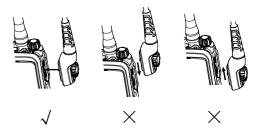
3. Tighten the screw on the accessory plug.
