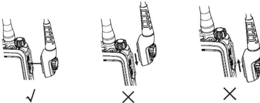
**Step 3** Tighten the screw on the accessory plug.
