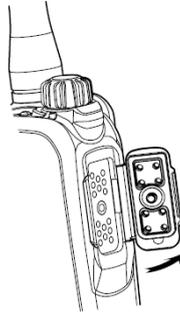
**Step 2** Align the accessory (such as an audio accessory or a programming cable) plug with the accessory connector.
