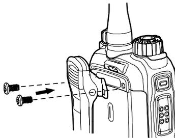
**Step 3** Tighten the screws.
