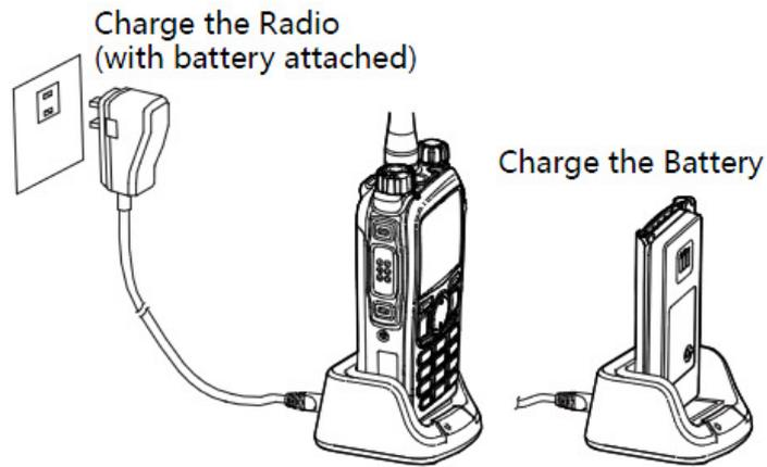
The LED indicator on the charger shows the charging status. For details, see the following table.
