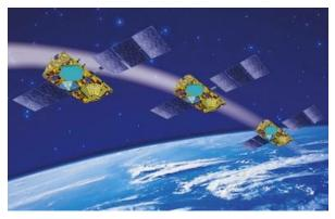
Messages are transmitted from the SmartOne via the Globalstar Satellite Network using an uplink-only connection (one-way data transmission) and received by a Globalstar Ground Station. The messages are then sent via an HTTP or FTP server to the internet and received by the VAR or end customer's back office application and converted into actionable data.
