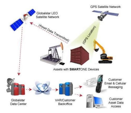
The SmartOne has the unique ability to check its GPS coordinates at a programmable rate while it is inside of the Change of Location Area without actually sending a message over the Globalstar Satellite Network.
