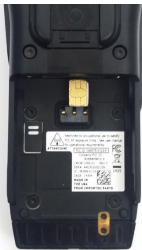
Figure 4-4: SIM Card Installation
