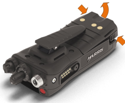
Figure 4-2: Remove the Battery
