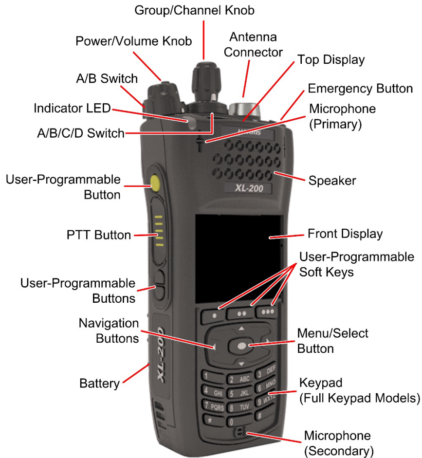
Figure 5-1: Radio Controls
