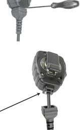
4. Insert the small flathead screwdriver under the locking tab of the RJ45 connector and push the tab up.  $_{<\!<\!<}$
