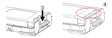
**Step 3** Push the battery until it is fully fitted into the slot, and then release the battery latch as ④ shows.
