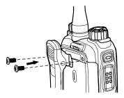
Step 3 Tighten the screws.
