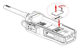
**Step 3** Replace the cover and tighten the screw as shown below.
