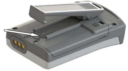
Insert the clip blade tool or similar device under the edge of the media as indicated by the arrow and lift it from the pager body. Once the stand is removed, gently slide the clip down the pager until it releases from the main body.
